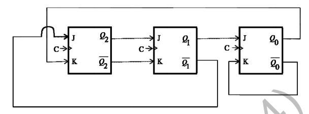
The above synchronous sequential circuit built using JK flip-flops is initialized with  $Q_2Q_1Q_0=000$ . The state sequence for this circuit for the next 3 clock cycles is
